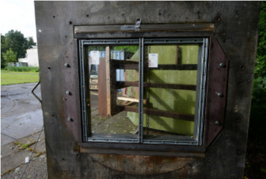
Specimen seen from the exposed side at the blast test facility with another type of glass. This picture is used to show the construction of the window frame itself.
