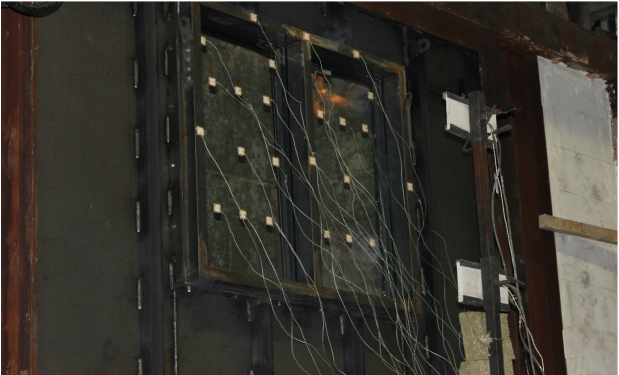
InterDam G21 Fire Window during fire post blast test
