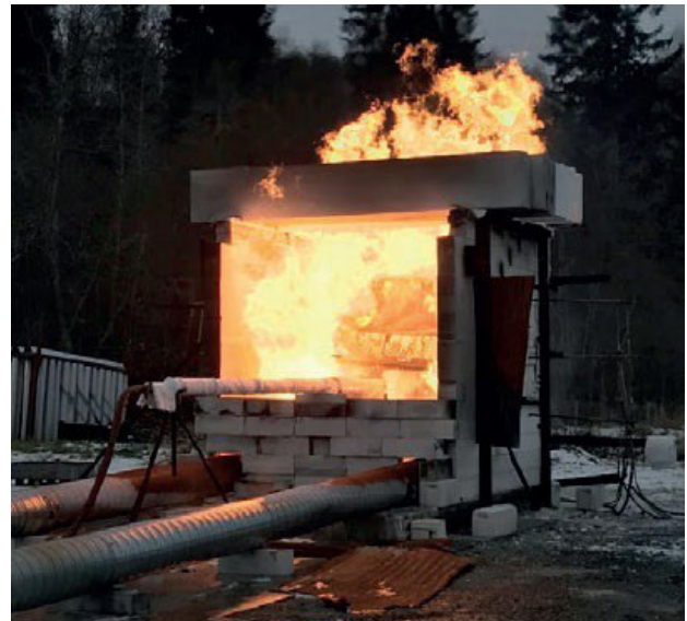
Figure: J15 HHF test on Norsok approved sliding door
